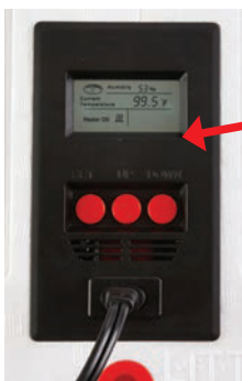
Digital readout of temperature and humidity levels
